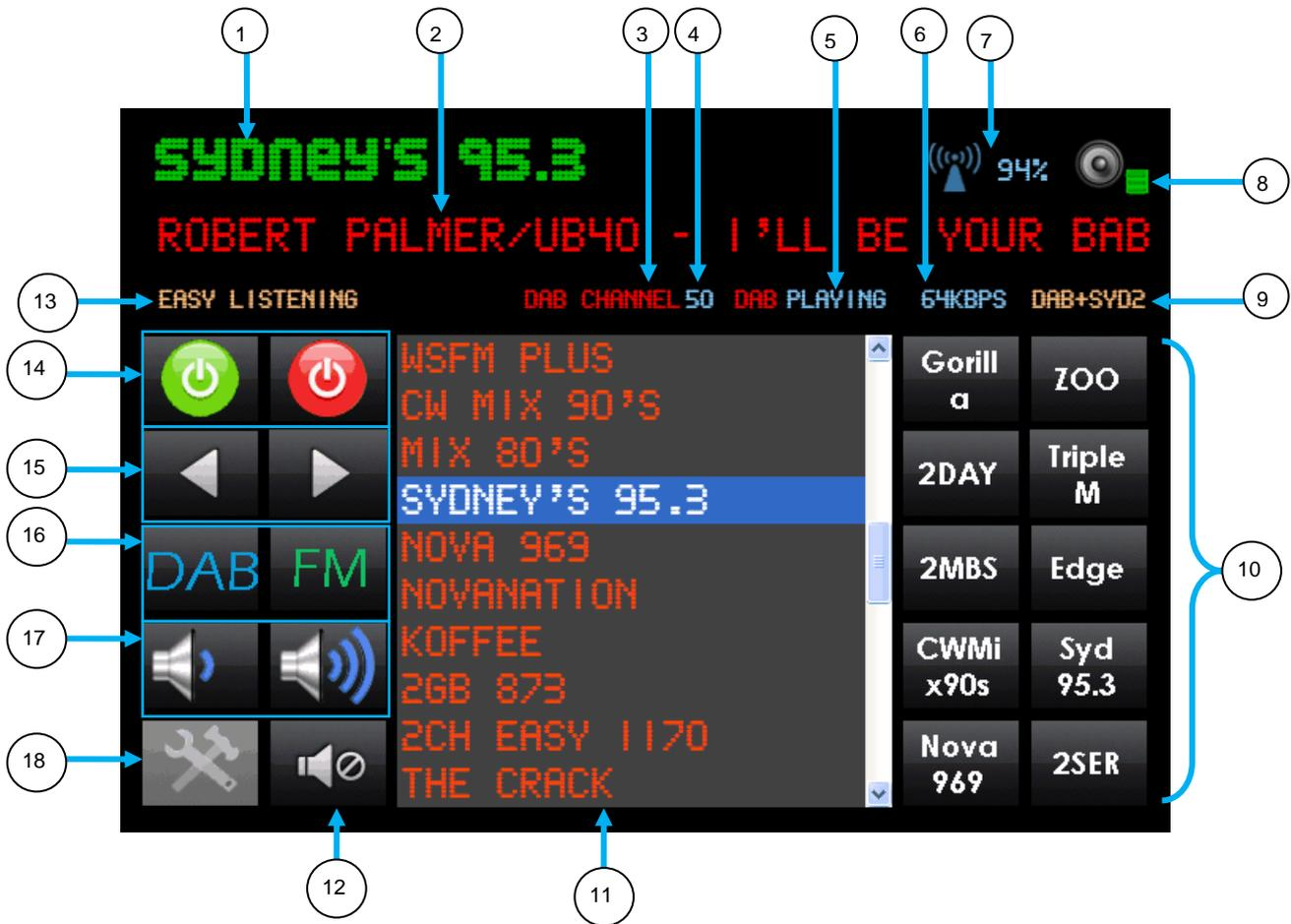
Figure 2.7: Basic Navigation and Function of each Button
